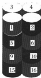
图 2 测试试件温度的均匀性的单元法 Fig. 2 The unit method to test the temperature uniformity of concrete specimens
